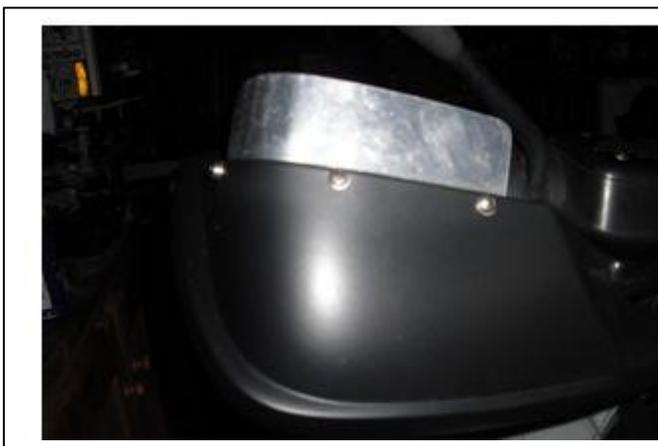
However, at £20 for two bits of plastic and £8.40 postage I decided to make my own! Fortunately there was some aluminium scrap at work and, after a bit of cutting with a guillotine and bending in a vice, plus nuts and bolts from the bin, I got my extensions done for zero pence! Hopefully the heated grips will be much more effective now and after fixing a broken connector on my heated waistcoat I am ready for winter. Time will tell!
